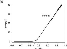
**Fig. 9** a) The Vis-NIR solid-state diffuse reflectance spectrum of (7)(TCNQ). b) The Tauc plot derived from the spectrum indicating the estimation of the optical band gap.
