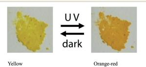
Fig. 2 Color change of I before and after UV irradiation.
