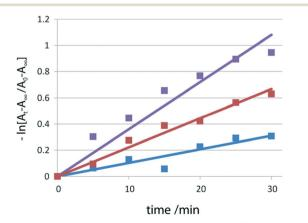
Fig. 6 Fading rates of I before visible-light irradiation (blue), and after 4 min (red) and 15 min (violet) irradiation.
