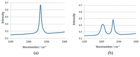
Fig. 4 Change in IR spectra of I (a) before and (b) after 120 min visible-light irradiation. The stretching vibration modes of the 2-ce and 1-ce groups appear at 2240 and 2200 cm<sup>-1</sup>, respectively
