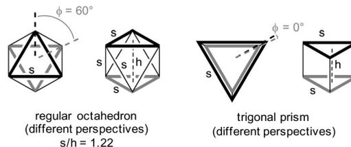
**Scheme 4** Octahedron and trigonal prism with enhanced triangular faces and relevant parameters for the assessment of their relationship.  $\phi$  is the twist angle between the enhanced triangles around the C<sub>3</sub> axis.
