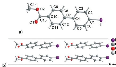
**Fig. 1** (a) Asymmetric unit (50% thermal ellipsoids) and (b) projection of the unit cell packing of 2. Selected distances (Å) and angles ( $^\circ$ ): C1–I1 2.082(9), C13–O1 1.202(13), C13–O2 1.303(12), O1–C13–C10 123.4(9), O1–C13–O2 123.6(10).
