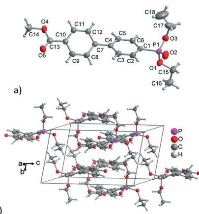
Fig. 2 (a) Asymmetric unit (50% thermal ellipsoids) and (b) crystal packing in **3**. Selected distances ( $\text{\AA}$ ) and angles ( $^\circ$ ): P1–O1 1.560(2), P1–O2 1.462(2), P1–O3 1.567(2), C13–O5 1.195(3), C13–O4 1.341(3), O1–P1–O2 116.11(13), O2–P1–O3 113.98(13), O1–P1–O3 102.44(13).
