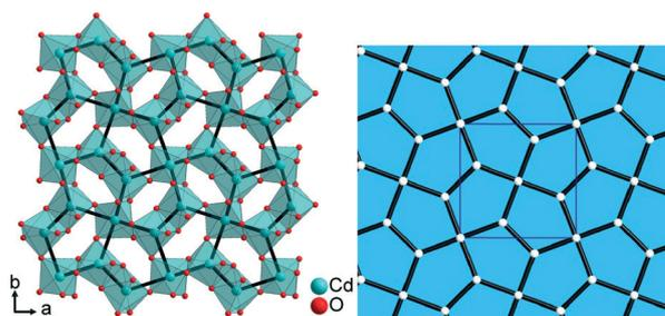
**Fig. 6** Left: Layer of {CdO<sub>6</sub>} polyhedra in 7 with the Cd atoms connected by black lines to illustrate the pentagonal *mcm* tiling. Right: *mcm* net from <http://rcsr.net/layers/mcm>.<sup>79</sup>
