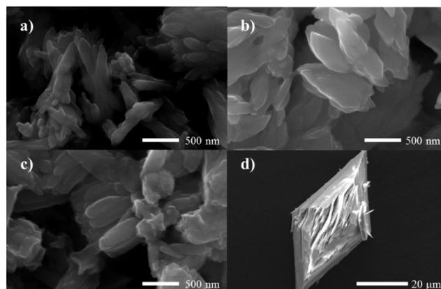
Fig. 2 SEM images of crystals of 1 prepared at room temperature using a reaction solution containing 0.1 M NaOH over a) 0.5 h and b) 16 h, or c) with  $\text{Na}_2\text{bcppm}$  over 16 h, and d) a conventional preparation over 16 h.
