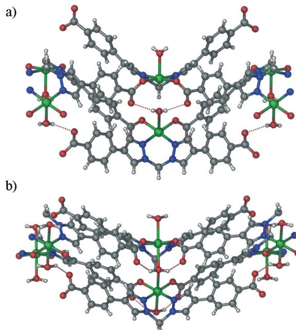
Fig. 4 The coordination environment of copper(II) centres in a) 1-S and b) 1, where the dotted red lines denote hydrogen bonding.<sup>34</sup> Green, grey, blue, red and white spheres represent Cu, C, N, O, and H atoms, respectively.
