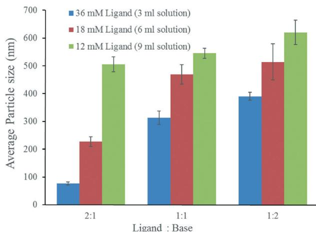
Fig. 3 Average particle size of 1b-S after 0.5 h by altering the concentration of H<sub>2</sub>bcp<sup>pm</sup> and the ligand to base ratio from 2:1 to 1:1 and 1:2.
