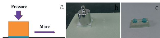
Fig. 16 (a) Schematic diagram of the abrasion test; (b) photo of abrasion test and (c) water droplets exhibiting a spherical shape on the scratch surface.
