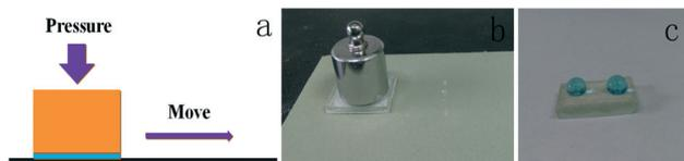
Fig. 16 (a) Schematic diagram of the abrasion test; (b) photo of abrasion test and (c) water droplets exhibiting a spherical shape on the scratch surface.
