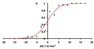
Fig. 6 Relationship between  $\Delta G_i^{\circ}$  and  $p_i$  obtained by summing H-bond populations over 2 kJ mol<sup>-1</sup> windows in  $\Delta G_i^{\circ}$  (RMSE = 0.07). The red line corresponds to the Boltzmann distribution in eqn (5).
