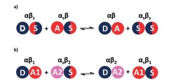
Fig. 1 (a) Formation of a H-bonded complex between two solutes in solution is determined by the equilibrium between solute-solvent interactions in the free state and solute-solute (A·D) and solvent-solvent (S·S) interactions in the bound state. (b) Competition between two different H-bond acceptors (A1 and A2) for one H-bond donor (D) in solution. The energy of each pairwise interaction can be estimated as the product of the relevant H-bond parameters.
