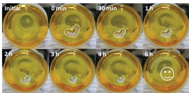
Fig. 2 Self-healing process of the PIL@PAA-Azo organogel.
