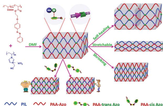
Scheme 1 Schematic illustration of preparation of a PIL@PAA-Azo organogel and its versatile performances.
