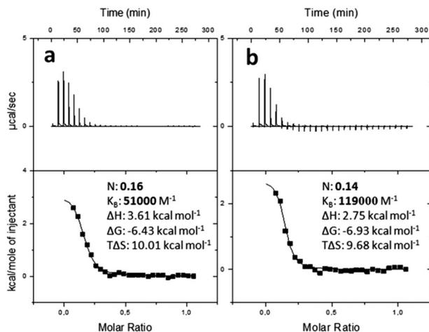
Fig. 4 Heat effects measured using ITC in the titration of PAA-Azo by PIL in traditional mode: (a) PAA-Azo solution before UV irradiation; (b) PAA-Azo solution after UV irradiation ( $N$ , stoichiometric ratio;  $K_B$ , binding affinity;  $\Delta H$ , enthalpy;  $\Delta G$ , free energy;  $T\Delta S$ , entropy).
