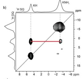
Fig. 2 (a) <sup>1</sup>H (400.23 MHz) MAS SSNMR spectra of the starting reagents and  $xKNH_2 + (1 - x)KH$  samples at different compositions (x = 0.1, 0.5, 0.9) after annealing recorded with a spinning speed of 32 kHz. Asterisks denote impurities. (b) 2D <sup>1</sup>H (400.23 MHz) DQ MAS SSNMR spectrum of the  $KNH_2 + KH$  (x = 0.5) after annealing recorded with a spinning speed of 32 kHz. The red line highlights the DQ correlation between the KH and KNH<sub>2</sub> signals.
