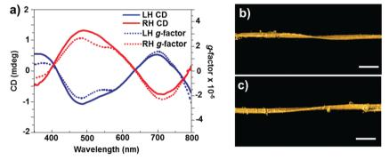
Fig. 5 (a) CD (solid line) and g-factor (dotted line) spectra for solutions of left- and right-handed nanoribbons obtained after 50 h of illumination with circularly polarized light. (b and c) Representative 3D TEM tomographic reconstructions of left- (b) and right-handed (c) nanoribbons. Scale bars = 100 nm. Adapted with permission from ref. 76. Copyright 2015 Nature Publishing Group.
