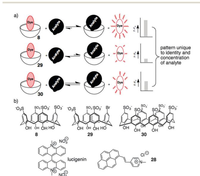
**Fig. 13** (a) Schematic representation of a chemical sensor array based on indicator displacement. (b) Sensor array components: calixarenes **8**, **29**, and **30** were combined with either lucigenin or dye **28** to create three-element sensor arrays for analysis of post-translationally modified amino acids and peptides.
