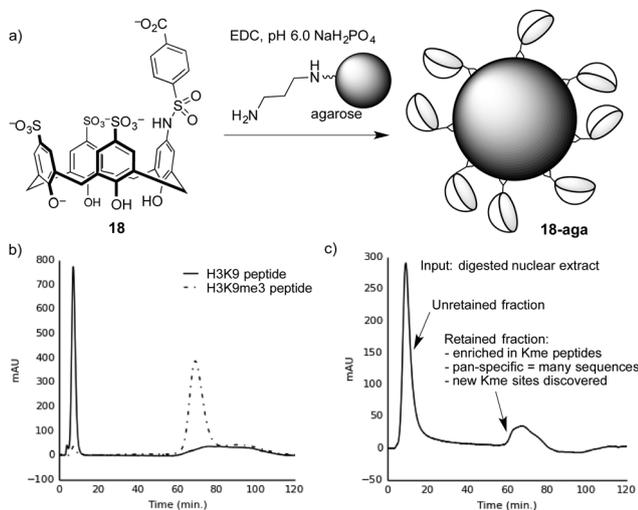
**Fig. 16** (a) Preparation of a trimethyllysine-binding stationary phase. (b) A chromatogram showing selective retention by stationary phase **18-aga** of a trimethyllysine-containing peptide over an unmethylated analog. (c) Chromatogram resulting from separation of a proteolyzed extract containing dozens of nuclear proteins on **18-aga**. The results from proteomics analysis of the retained material<sup>86</sup> are summarized.
