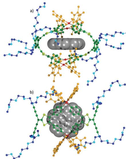
Fig. 3 X-Ray crystal structure of coronene in  $M_4L_2$  (a) side view, (b) top view. Colors used: exTTF skeleton (green), PEG chains (blue), Pd complex (orange), coronene (grey).
