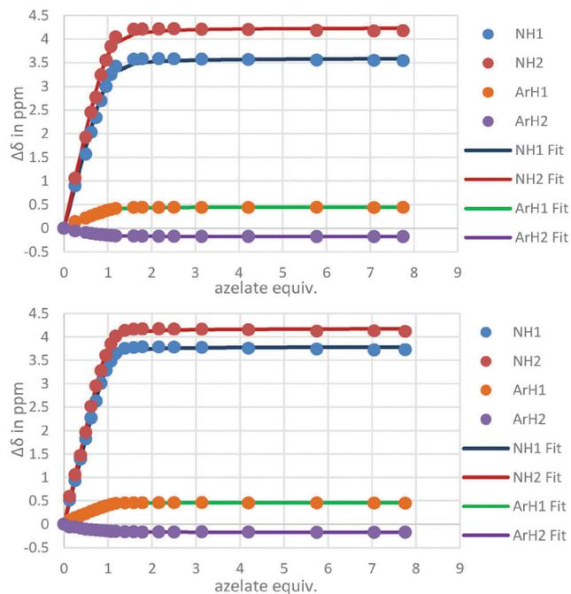
**Fig. 2** Isotherms resulting from the <sup>1</sup>H NMR titrations of hosts **1** and **2** with azelate (C9).
