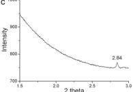
Fig. 2 (a) TEM image of the SOF fabricated from 1 (0.0125 mM) and CB[8] (0.0188 mM), (b) tapping-mode AFM image and section analysis of the SOF fabricated from 1 (0.0125 mM) and CB[8] (0.0188 mM), and (c) synchrotron SAXS profiles of the SOF obtained by evaporating its solution. The SOF was prepared by dissolving a mixture of 1 and CB[8] (2:3) in water-methanol (17:3, V/V) and standing overnight without disturbance at room temperature.
