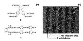
**Fig. 5** (a) Molecular structures of **1** and **2** (b) optical polarized light microscope image of a patterned sample of **1**, **2** at 65 °C prepared by cooling under UV light using a photomask. Adapted from ref. 73 with permission from the Royal Society of Chemistry.
