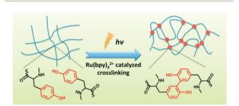
**Fig. 19** Irradiation of a tyrosine-containing LMWG in the presence of a ruthenium catalyst leads to cross-linking and a dramatic increase in gel strength. Reproduced from ref. 135 with permission of the Royal Society of Chemistry.
