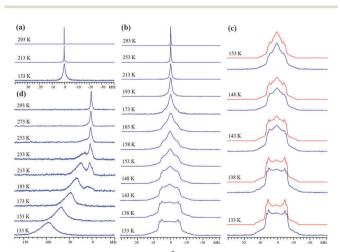
Fig. 1 The experimental static VT <sup>2</sup>H SSNMR spectra of adsorbed D<sub>2</sub> within (a) Zn-MOF-74, (b and c) Mg-MOF-74, and (d) Ni-MOF-74 are depicted. Experimental (blue) and simulated (red) <sup>2</sup>H SSNMR spectra in Mg-MOF-74 at low temperatures are shown in (c). The sharp resonance at ca. 0 kHz in all spectra at high temperatures corresponds to mobile or very weakly adsorbed D2; this resonance is broadened in (d) due to the influence of the paramagnetic Ni metal center.
