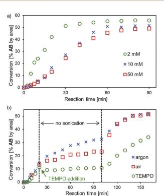
Fig. 3 HPLC monitoring of the metathesis of disulfides AA and BB under sonotrode conditions in chloroform. (a) Influence of starting material concentration (2 mM, 10 mM, 50 mM). (b) Influence of switching off the ultrasound source (period: 20-100 min) in argon, air or in argon with addition of 40 mM of radical scavenger TEMPO ((2,2,6,6-tetramethylpiperidin-1-yl)oxyl) after 20 min.
