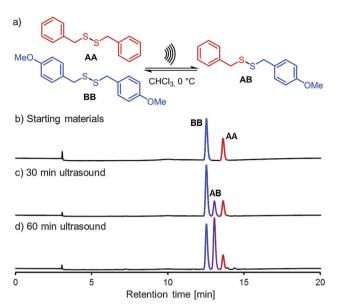
Fig. 2 (a) Ultrasound-induced disulfide metathesis. Reaction conditions: AA (10 mM) and BB (10 mM), sonotrode irradiation (25% amplitude, pulse sequence 0.5 s on, 1.0 s off), CHCl $_3$ , 0 °C. (b) Analytical HPLC (70%  $\rightarrow$  100% gradient acetonitrile/water, 0.3 mL min<sup>-1</sup>, Ascentis amide column) of starting materials AA and BB. (c) Analytical HPLC after 30 minutes of sonication. (d) Analytical HPLC after 60 minutes of sonication.
