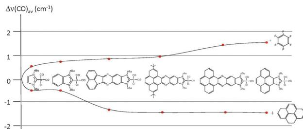
**Fig. 6** Representation of the variation of the average C–O stretching frequencies of a series of  $[\text{IrCl}(\text{NHC})(\text{CO})_2]$  complexes. The data were taken from the IR spectra of the complexes in  $\text{CH}_2\text{Cl}_2$ , by adding 5 equivalents of the additive (pyrene or hexafluorobenzene). Solid lines are used only to guide the eye.
