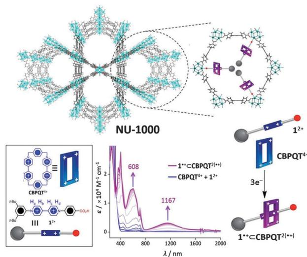
Fig. 5 Schematic of NU-1000 containing the semirotaxane (top). Representation of the semirotaxane components  $1^{2+}$  and  $CBPQT^{4+}$  (bottom left). Reduction of  $1^{2+}$  and  $CBPQT^{4+}$  with 3 mol  $e^-$  generates the semirotaxane  $1^+ < CBPQT^{2(+)}$  (bottom right and centre where the redox-dependent absorption spectrum is shown). Reproduced from ref. 148 with permission from National Academy of Sciences, USA.
