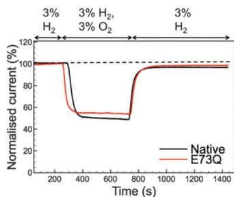
**Fig. 3** Inhibition and recovery from 3% O<sub>2</sub> measured at +0.113 V vs. SHE with 3% H<sub>2</sub> throughout. The black line shows data for Native *Escherichia coli* Hyd-1 while the red line depicts the measurement for the E73Q variant. Other experimental conditions: pH 4.5; 37 °C; electrode rotation rate 3500 rpm; carrier gas N<sub>2</sub> and total gas flow rate 100 scc min<sup>-1</sup>.
