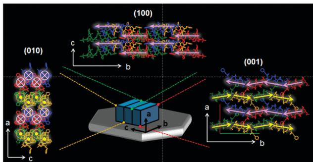
Fig. 4 The complete molecular arrangement of foldecture **P**<sub>1</sub>. A blue box representing a unit cell is laid on the hexagonal plate (gray) alongside the absolute axes. Extended molecular networks ( $2 \times 2 \times 2$ ) as viewed along the *a*- (top), *b*- (left), and *c*-axes (right) show the molecular-level packing. The pink and yellow arrows and symbols ( $\odot$  and  $\otimes$ ) superimposed on each foldamer indicate the helical direction (N to C).
