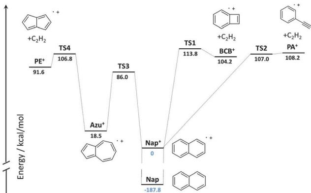
Fig. 1 Summary of the possible  $C_2H_2$  loss channels on the  $C_{10}H_8^+$  potential energy surface constructed from the data reported in Dyakov *et al.*<sup>17</sup>
