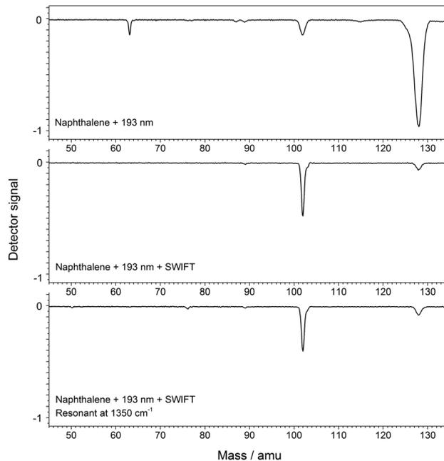
Fig. 2 Mass spectra of naphthalene dissociatively ionized at 193 nm (top trace), the SWIFT isolated fragment at  $m/z = 102$  (middle trace) and the SWIFT isolated fragment dissociated with intense IR radiation at  $1350\text{ cm}^{-1}$ .
