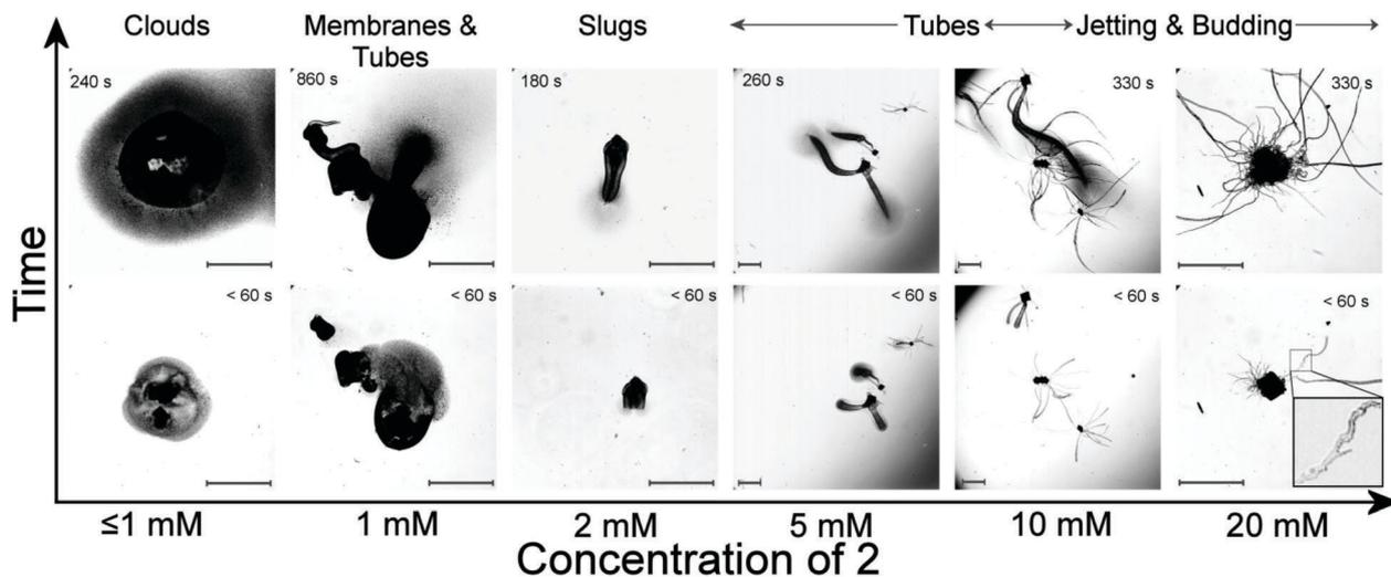
Fig. 3 The range of precipitation structures observed for the polyoxometalate–polyoxocation system described here, ranging from cloud like structures at low concentrations to jetting and budding tubes at higher concentrations. Inset on lower 20 mM figure highlights the budding growth regime. Scale bars = 400  $\mu\text{m}$ .
