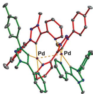
Fig. 2 Ortep drawing (30% probability ellipsoids) of cation **1'** (blue = N, gray = C, and violet = Pd) with bidentate (green) and bridging coordination (red). Anions, solvents and hydrogen atoms are omitted for clarity (ESI†).
