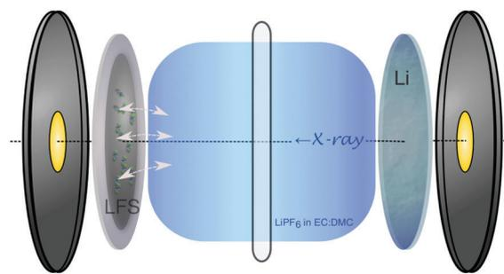
Fig. 1 Schematic of the *in situ* CR2032 coin cell with Kapton<sup>®</sup> windows used for XANES monitoring of the LFS–electrolyte interaction (depicted with arrows at the solid–electrolyte interphase).
