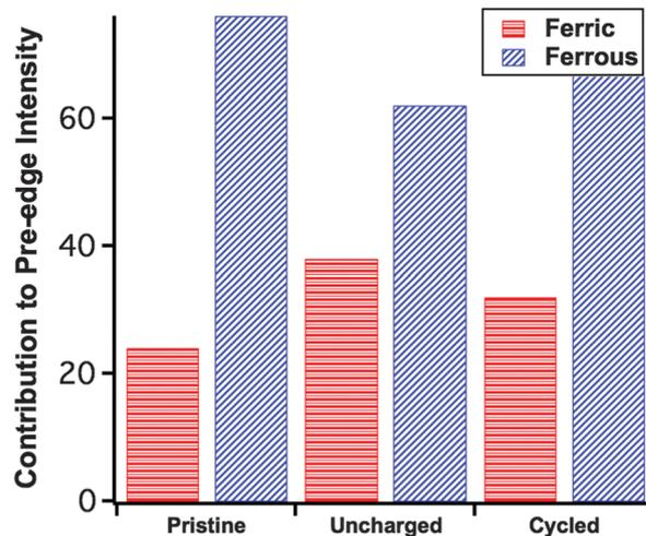
Fig. 4 Category plot of the Fe<sup>2+</sup> and Fe<sup>3+</sup> contribution to the pre-edge for the pristine material, uncharged (20C<sub>0</sub>) and cycled (20D<sub>f</sub>), as determined by a linear combination fit with FeS<sub>4</sub> reference compounds: low-temperature XAS from molecular FeS<sub>4</sub> in rubredoxin.
