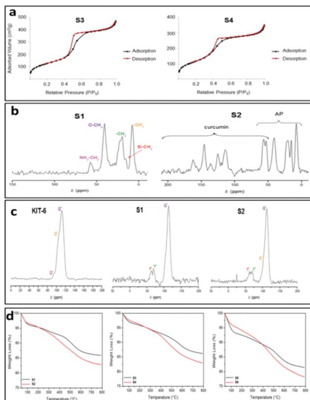
**Fig. 1** (a) Nitrogen adsorption–desorption isotherms of materials **S3** and **S4**. (b)  $^{13}\text{C}$ -CP MAS NMR spectra of materials **S1** and **S2**. (c)  $^{29}\text{Si}$  MAS NMR spectra of materials **KIT-6**, **S1** and **S2**. (d) Thermogravimetric analysis of materials **S1–S6**.
