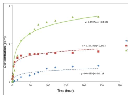
**Fig. 3** Release study of curcumin present in S2, S4 and S6 in Tris-HCl (pH 7.4). The results show the slow and sustained release of curcumin from the materials. The error bars are omitted for clarity.
