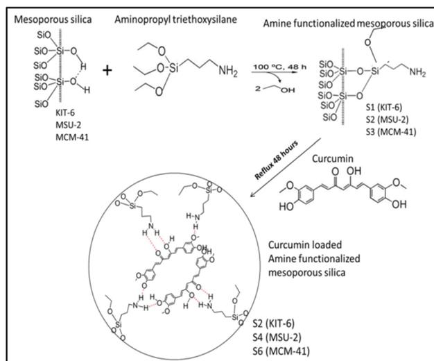
**Scheme 1** Synthesis of mesoporous silica based materials **S1**–**S6**. Amine functionalization of starting materials KIT-6, MSU-2 and MCM-41 with 3-aminopropyltriethoxysilane (APTES) generates **S1**, **S3** and **S5**. The reaction of these materials with curcumin under nitrogen atmosphere forms the curcumin loaded materials **S2**, **S4** and **S6**, respectively.
