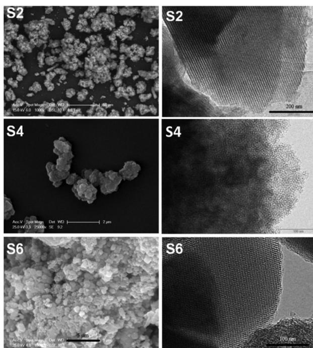
**Fig. 2** Electron microscopy images of materials S2, S4 and S6. The SEM images show that the morphology and arrangement of the materials are maintained as in the corresponding starting materials. TEM images exhibit pore arrangements of the materials similar to those found in the starting materials.
