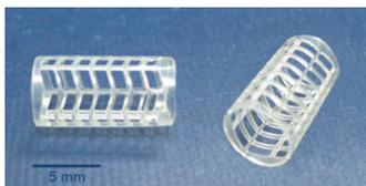
**Fig. 8** A prototype stent fabricated from a high molecular weight poly(LLA-co-GA-co-TMC) (LLA/GA/TMC = 95/5/5). Reprinted with permission from ref. 151. Copyright (2013) Society of Plastics Engineers.
