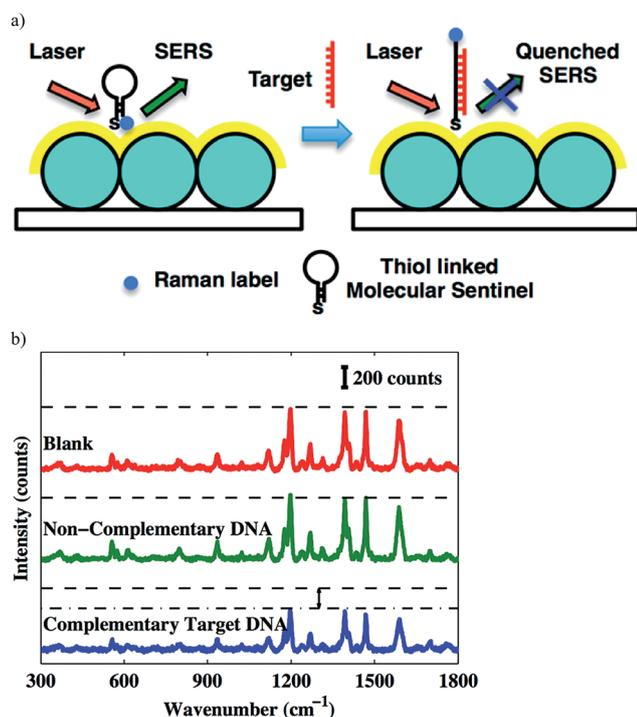
Fig. 7 (a) Detection scheme of the complementary target DNA; (b) SERS spectra. Notice the decreasing signal intensity due the presence of target DNA.<sup>65</sup> Copyright © 2013, American Chemical Society.
