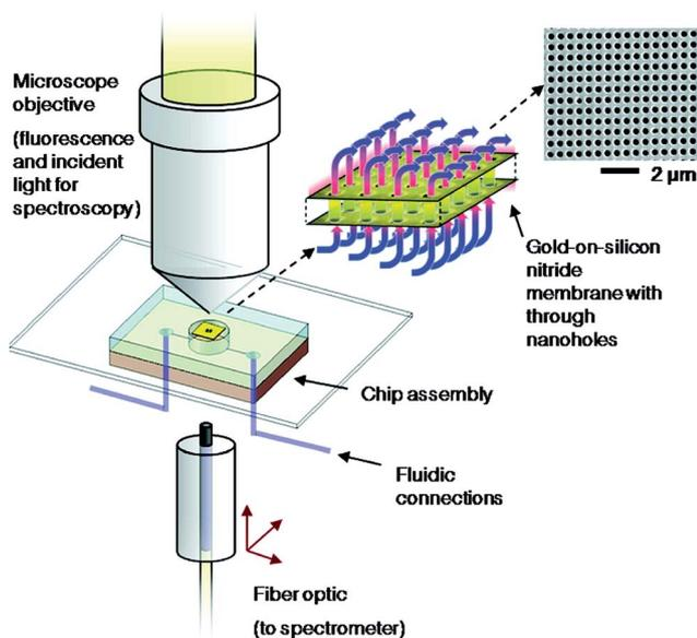
Fig. 12 Flow-through nanohole arrays biosensing scheme developed by Brolo group. Reproduced with permission.<sup>102</sup> Copyright © 2009, American Chemical Society.
