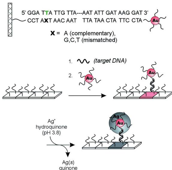
Fig. 6 Three-component scanometric assay for specific oligonucleotide detection reported by Mirkin group. Reproduced with permission.<sup>61</sup> Copyright © 2000, The American Association for the Advancement of Science.
