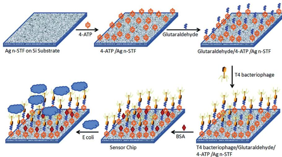
Fig. 15 Schematic illustration for *E. coli* biosensor-chip development. The chip of silver nSTFs over a Si substrate is modified with a SAM of 4-aminothiophenol (4-ATP). This SAM is further modified with glutaraldehyde for phage immobilization. BSA is added to block unreacted glutaraldehyde. The chip is exposed to the sample and monitored using a fiber optic Raman spectrometer. Reproduced with permission.<sup>117</sup> Copyright © 2015, Royal Society of Chemistry.
