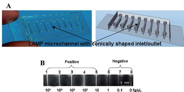
**Fig. 1** (A) Eight-channel PDMS–glass hybrid microfluidic chip for LAMP: (left) photograph and (right) schematic drawing of an eight-channel PDMS–glass hybrid microfluidic chip. (B) Sensitivity of LAMP using direct visual detection. Channels 1–5 show the white precipitate (channels appear white), while channels 6–8 do not (channels appear dark). Reproduced with permission.<sup>27</sup> Copyright © 2010, American Chemical Society.
