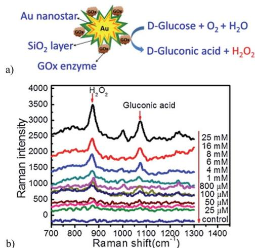
**Fig. 18** (a) Scheme illustration of glucose detection by the Au nanostar@silica core-shell nanoparticles based SERS sensor. (b) SERS spectra shown the Raman enhancement when the concentration of glucose is increased. Reproduced with permission.<sup>125</sup> Copyright © 2011 Elsevier B.V.
