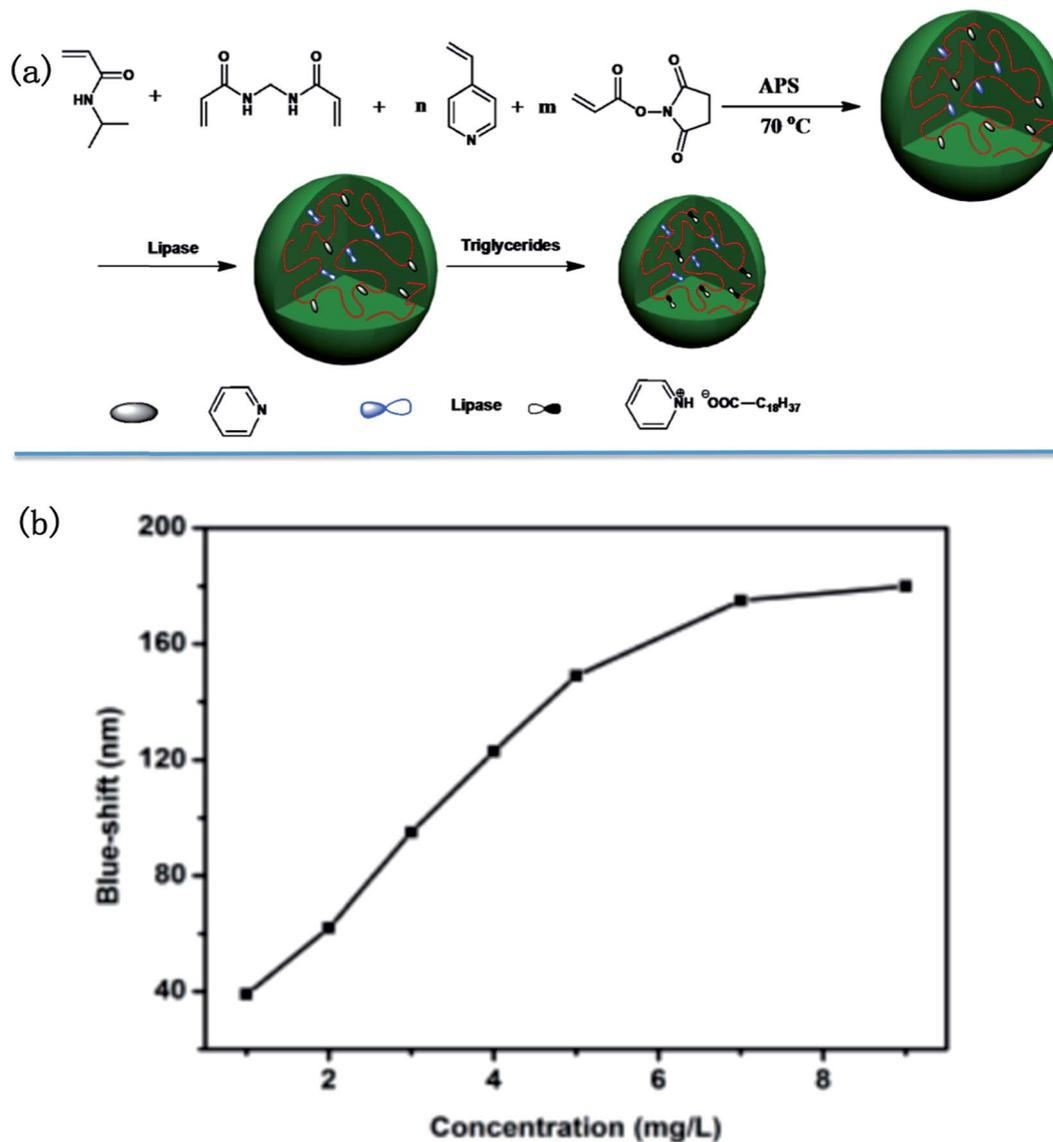
Fig. 17 (a) Microgel synthesis scheme; (b) blue-shift as function of triglyceride concentration. Reproduced with permission.<sup>121</sup> Copyright © 2015, Royal Society of Chemistry.
