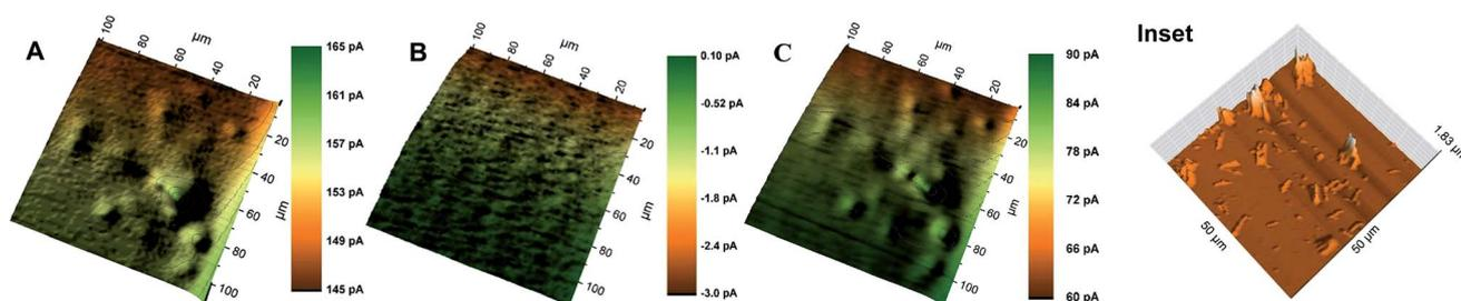
Fig. 6 SECM images of HRP-linked AuNW clusters immobilized on a gold-coated glass slide at (A) 0.3 V probe potential (positive feedback), (B) 0 V probe potential, and (C) 0 V probe potential after the addition of 0.3% H<sub>2</sub>O<sub>2</sub> (SG/TC). The images were recorded with Pt probes of radii 1–3  $\mu\text{m}$  at a scan rate of 50  $\mu\text{m s}^{-1}$  in 1.5 mM ferrocenemethanol solution in pH 6 SPB. Inset: representative AFM image of the same substrate.
