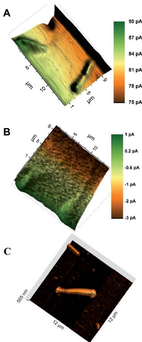
Fig. 7 SECM images of individual HRP-linked AuNWs immobilized on a gold-coated glass slide at (A) 0.3 V probe potential (positive feedback) and (B) 0 V probe potential after the addition of 0.3%  $\text{H}_2\text{O}_2$  (SG/TC). The images were recorded with a 300 nm radius probe at a scan rate of  $5\ \mu\text{m s}^{-1}$  in 1.5 mM ferrocenemethanol solution in pH 6 SPB. (C) Representative AFM image of the same substrate.
