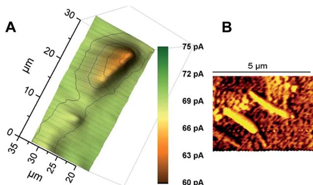
Fig. 2 (A) Negative feedback SECM image of individual AuNWs immobilized on a glass slide. The image was recorded with a  $300 \text{ nm}$  radius Pt probe at a potential of  $0.3 \text{ V}$  and a scan rate of  $5 \mu\text{m s}^{-1}$  in  $1.5 \text{ mM}$  ferrocenemethanol solution. (B) Representative AFM image of AuNWs immobilized on a glass slide.
