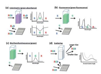
Fig. 2 Typical optical detection for both light transmitted through liquid sample platforms (*i.e.* cuvette, well plate) and light reflected from solid sample platforms (*i.e.* test strip, cassette) using (a) colorimetric assays, (b) fluorescence-based assays, (c) bio- and chemiluminescence assays, and (d) scattering-based assays.
