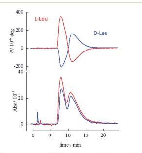
Fig. 3 Chiral separation of BINOL with frozen 5.0 mM Leu, with pH adjusted to 11. The upper and lower chromatograms were recorded simultaneously through CD and UV detection, respectively. Mobile phase: 5% (v/v) diethyl ether/n-hexane; temperature: -8.0 °C.
