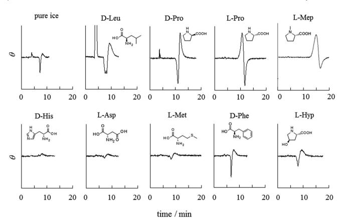
Fig. 1 Screening of frozen amino acids for chiral resolution of BINOL. All of the stationary phases were prepared by freezing 5.0 mM amino acids. Mobile phase: 5% (v/v) diethyl ether/n-hexane; temperature: -8.0 °C.
