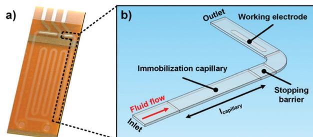
**Fig. 2** (a) Photograph of the standard microfluidic biosensor fabricated by dry film photoresist technology with (b) the inset depicting the simulation model and its main features: immobilization capillary, working electrode and stopping barrier.
