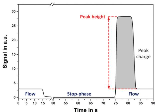
**Fig. 1** Typical signals obtained from a stop-flow measurement. For the data evaluation, either the maximum height or the charge of the rectangular-shaped peak signal can be utilized. Both signal parameters are proportional to the period of the stop-phase.
