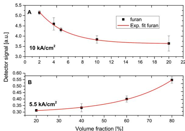
Fig. 6 riQCL-iHWG sensor system response to furan (in 2-methoxyethanol) obtained *via* selective emission line damping at an applied voltage of  $10 \text{ kA cm}^{-2}$  (A), and of  $5.5 \text{ kA cm}^{-2}$  (B). An exponential fit was applied to the response function resulting in a calibration model with a coefficient of determination ( $R^2$ )  $>0.99$  for both curves.
