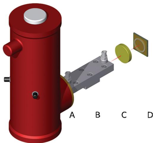
**Fig. 2** Prototype sensing setup comprising a HgCdTe semiconductor detector (A), an iHWG with 15 cm waveguide/gas cell channel length (B), a ZnSe lens for beam collimation (C), and a riQCL (D). In a next step, it is anticipated that the riQCL and the detector will be directly integrated into the iHWG structure. (Dimensions are not to scale).
