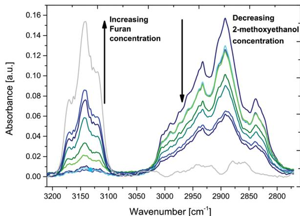
Fig. 5 For comparison, IR spectra were recorded by coupling an iHWG with  $7.5 \text{ cm}$  channel length to a conventional FT-IR spectrometer analyzing vapor phase samples with increasing concentrations of furan, and correspondingly decreasing concentrations of 2-methoxyethanol (0 to 100% for each constituent).
