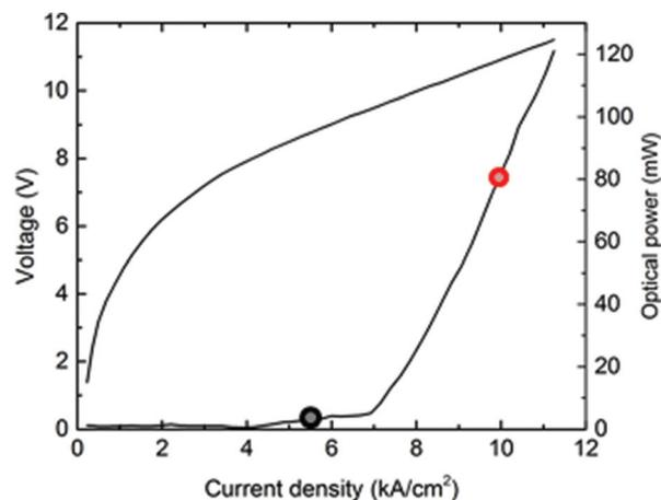
**Fig. 3** Voltage *vs.* current density curve of the riQCL representing the emitted optical output power operated at 293 K (room temperature) driving the riQCL either at 5.5  $\text{kA cm}^{-2}$  (●: emission wavelength @ 1144  $\text{cm}^{-1}$ ) or at 10  $\text{kA cm}^{-2}$  (●: emission wavelength @ 1144  $\text{cm}^{-1}$  and 1170  $\text{cm}^{-1}$ ).
