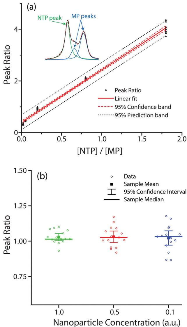
Fig. 5 (a) Linear regression of peak ratios of the  $1571\text{ cm}^{-1}$  and  $1597\text{ cm}^{-1}$  peaks, as a function of the molar ratio NTP:MP in probe adsorbate. Inset: Representative peak fitting; (b) scatter plot of peak ratios at various dilutions, including median, mean, and 95% confidence intervals.
