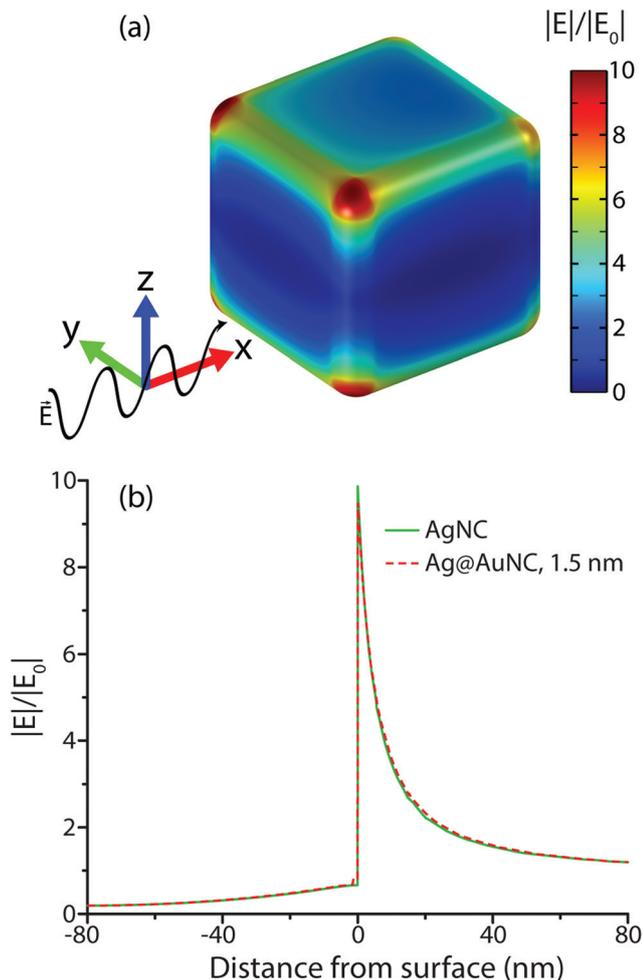
**Fig. 4** (a) Color map of the simulated electric field enhancement on the surface of a single Ag@AuNC with a 1.5 nm Au coat, suspended in water; (b) calculated electric field enhancement for AgNC and Ag@AuNC, measured along the [111] vector passing through the cube center.
