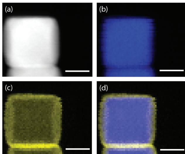
Fig. 2 (a) HAADF-STEM image of Ag@AuNC; (b) and (c) are the EDX elemental maps of Ag and Au, respectively. Blue represents the intensity of the Ag L<sub>α</sub> peak and yellow represents the average intensity of the Au L<sub>α</sub> and Au M<sub>α</sub> peaks; (d) combined elemental map of Ag and Au. All scale bars are 50 nm.
