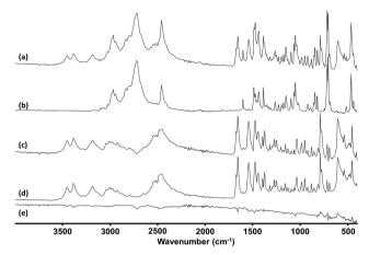
ATR-IR spectra of (a) a mixed seized sample. (b) MPA reference spectrum, (c) seized sample minus MPA reference, (d) lidocaine reference and (e) the residual spectrum after subtraction of both MPA and lidocaine. Spectra are vertically offset for clarity.
