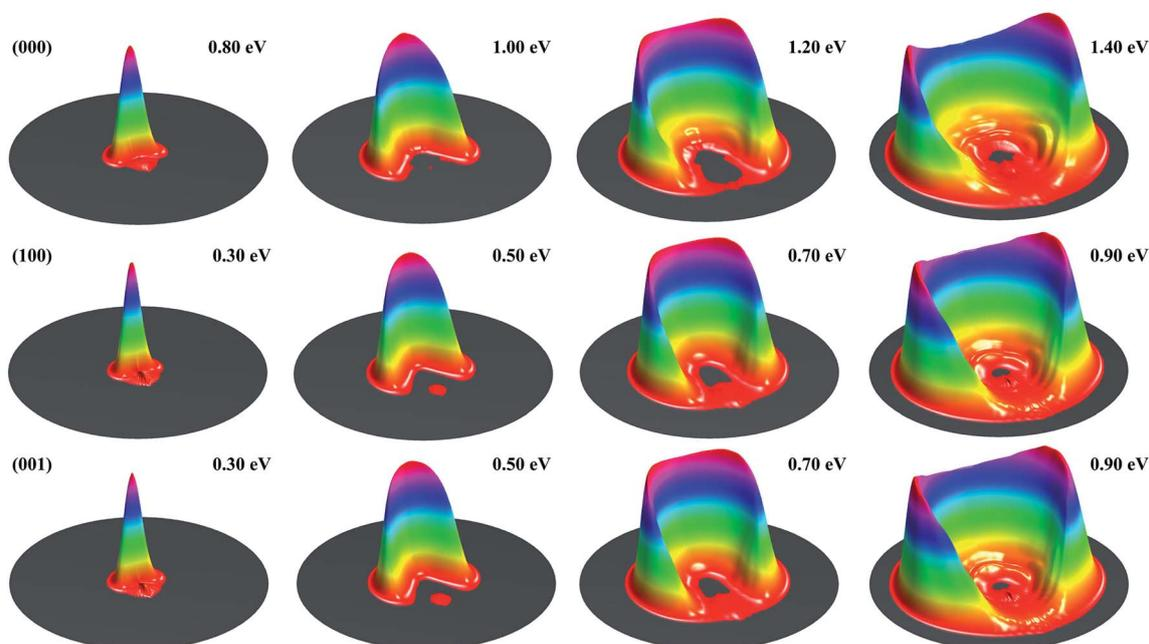
Fig. 1 Surface plots for the product translational energy and angle distributions for the three initial states (000), (100) and (001) at several collision energies.
