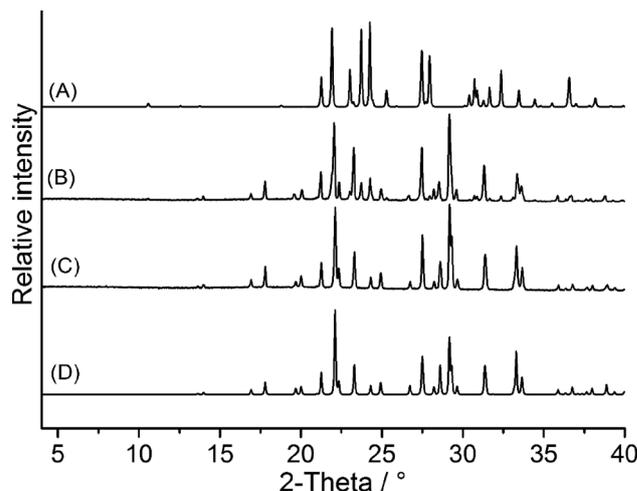
**Fig. 6** Experimental XRPD pattern of a mixture of form I and II (B) and of the residue after stirring this mixture in ethanol for one week (C) together with the calculated pattern for form I (A) and form II (D).
