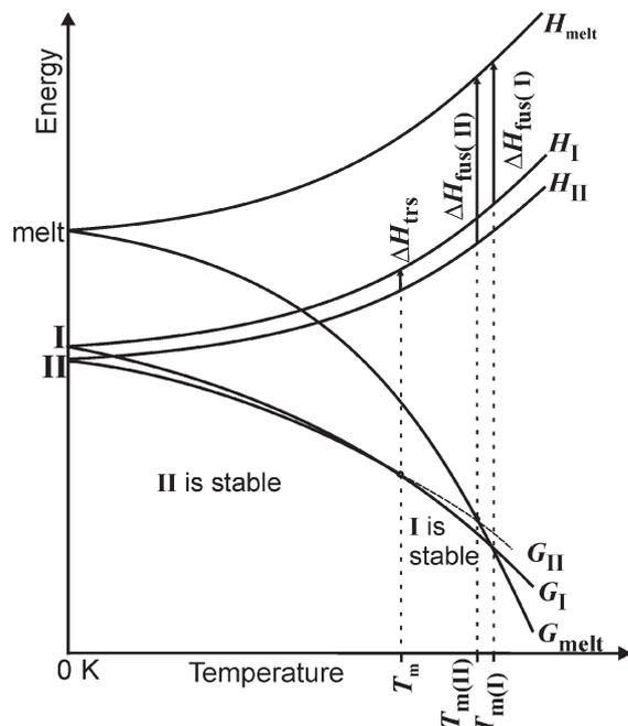
Fig. 10 Qualitative energy/temperature diagram for the enantiotropically related modifications I and II ( $G$  = free energy;  $H$  = enthalpy;  $T_{\text{trs}}$  = transition temperature;  $T_m$  = melting point;  $\Delta H_{\text{fus}}$  = enthalpy of fusion).
