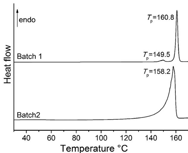
**Fig. 5** DSC curve of batch 1 (top) and batch 2 (bottom) at 10 °C min<sup>-1</sup>. Peak temperatures ( $T_p$ ) are given in °C.
