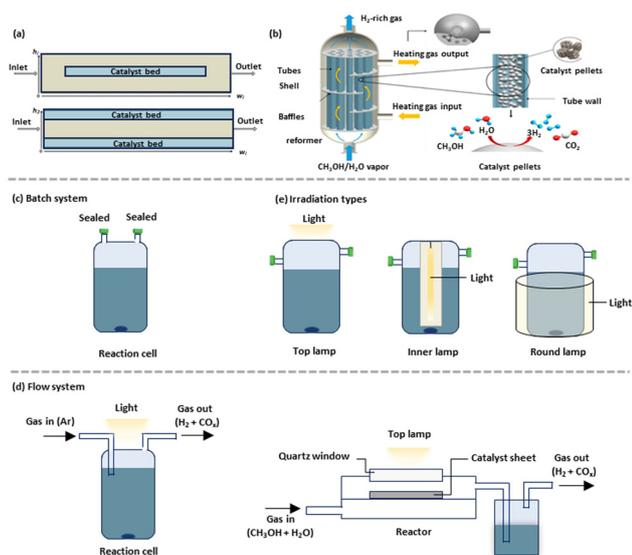
Fig. 6 Schematic representation of the reforming reactor: (a) packed bed and coated-wall packed bed microreactors, (b) a multi-tubular packed-bed reactor.<sup>184</sup> (c) Batch system and (d) flow systems. (e) The irradiation types. (b) Reproduced from ref. 184, no permission required.
