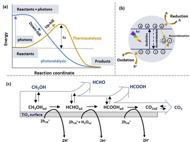
Fig. 2 (a) Difference in thermodynamics of photocatalysis and thermal catalysis. (b) Scheme for semiconductor photocatalysis. (c) The pathway for methanol oxidation on the TiO<sub>2</sub> surface.<sup>39</sup> (c) Reproduced from ref. 39 with permission from Elsevier, Copyright 2011.
