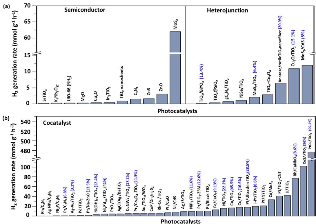
Fig. 3 Representative photocatalysts for methanol based H<sub>2</sub> production: (a) without cocatalysts or heterojunction structure and (b) loaded with different cocatalysts. The percentages highlighted in parentheses represent the quantum efficiency.
