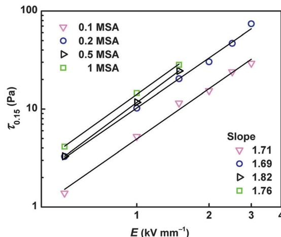
**Fig. 5** The double-logarithmic plot of shear stress values obtained at a shear rate of  $0.15 \text{ s}^{-1}$ ,  $\tau_{0.15}$ , vs. electric field strength,  $E$ , for the prepared ER fluids. The lines represent the exponential fit and their slope values involved in the graph.
