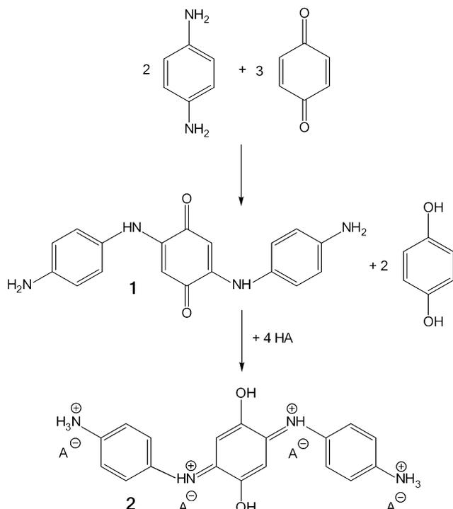
Fig. 1 *p*-Phenylenediamine is oxidized with *p*-benzoquinone to 2,5(di-*p*-phenylenediamine)-1,4-benzoquinone (1). After the “keto–enol” rearrangement, the resulting imine nitrogen atoms may become protonated with (methanesulfonate) acid (HA) to corresponding salt (2).
