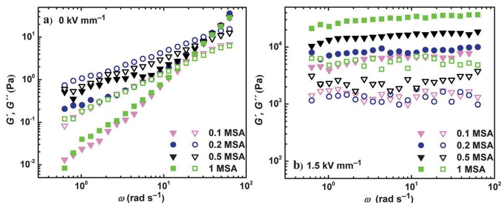
Fig. 7 The double-logarithmic plot of the storage,  $G'$  (solid symbols), and viscous,  $G''$  (open symbols), moduli vs. the angular frequency,  $\omega$ , for ER fluids based on DPB prepared in the presence of various MSA solutions in the absence (a) and in the presence of an electric field strength of  $1.5 \text{ kV mm}^{-1}$  (b).
