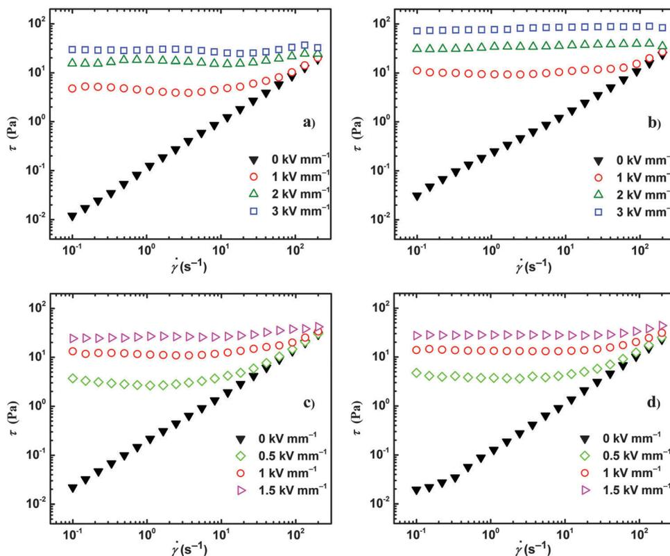
**Fig. 4** The double-logarithmic plot of the shear stress,  $\tau$ , on the shear rate,  $\dot{\gamma}$ , for the ER fluids based on DPB prepared in the presence of 0.1 M (a), 0.2 M (b), 0.5 M (c), and 1 M (d) MSA at various electric field strengths.
