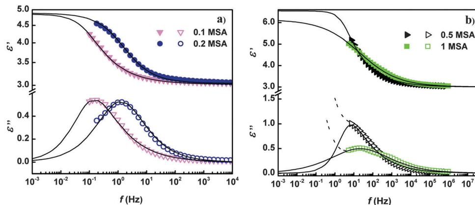
Fig. 8 Real,  $\epsilon'$ , (solid symbols) and imaginary,  $\epsilon''$ , (open symbols) parts of complex permittivity for the ER fluids based on DPB prepared in the presence of 0.1 M and 0.2 M MSA (a), and 0.5 M and 1 M MSA (b). The full lines represent the Havriliak–Negami model fits. The dashed lines represent original data indicating the electrode polarization that were excluded from fitting.
