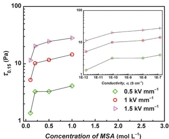
Fig. 6 The plot of shear stress values obtained at a shear rate of  $0.15 \text{ s}^{-1}$  vs. concentration of MSA presented during the synthesis of DPB for their 10 wt% ER fluids. The inset depicts shear stress values obtained at a shear rate of  $0.15 \text{ s}^{-1}$ ,  $\tau_{0.15}$ , vs. conductivity of the suspended particles.
