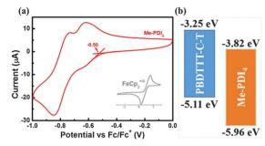
Fig. 4 (a) Cyclic voltammogram for Me-PDI<sub>4</sub> and (b) energy levels of the donor PBDTTT-C-T and the acceptor Me-PDI₄
