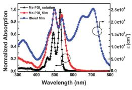
Fig. 3 UV-vis absorption spectra of Me-PDI<sub>4</sub> in solution, film and Me-PDIa: PBDTTT-C-T blend film.  $\varepsilon$ : refers to the absorption coefficient.
