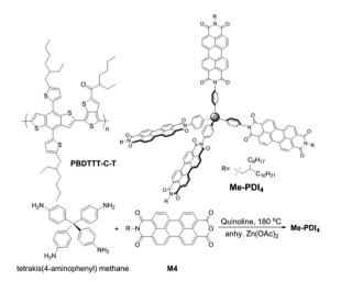
Scheme 1 Structure of PBDTTT-C-T and synthesis of Me-PDI<sub>4</sub>.
