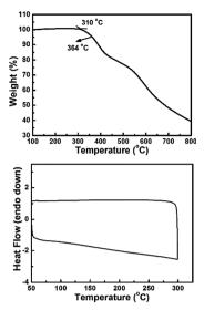
Fig. 1 TGA and DSC spectra of Me-PDI<sub>4</sub>.
