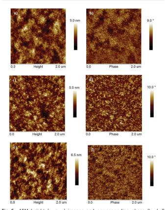
Fig. 6 AFM height (a, c, e) images and corresponding phase (b, d, f) images of PBDTTT-C-T:  $Me-PDI_4$  blend film treated without DIO (a, b), with 3% DIO (c, d) and with 3% DIO and 180 °C thermal annealing (e, f).
