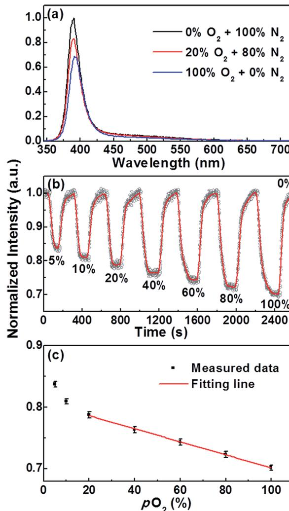
Fig. 4 (a) PL spectra of a TC NR sample measured at T<sub>NR</sub> = 150 °C in the presence of 100% N<sub>2</sub>, 20% O<sub>2</sub>/80% N<sub>2</sub> and 100% O<sub>2</sub>. (b) Dynamic I<sub>UV(max)</sub> response of the TC NR sample to various pO<sub>2</sub> at T<sub>NR</sub> = 150 °C. (c) I<sub>UV(max)</sub> from the TC NR sample measured as a function of pO<sub>2</sub> at T<sub>NR</sub> = 150 °C.
