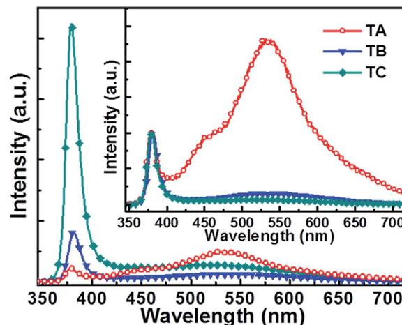
Fig. 2 PL spectra of ZnO nanorods grown with  $F \sim 4.0$  J cm<sup>-2</sup> (TA sample),  $\sim 1.8$  J cm<sup>-2</sup> (TB sample) and  $\sim 1.2$  J cm<sup>-2</sup> (TC sample). The inset shows the same PL spectra normalized to the same peak  $I_{UV}$ .
