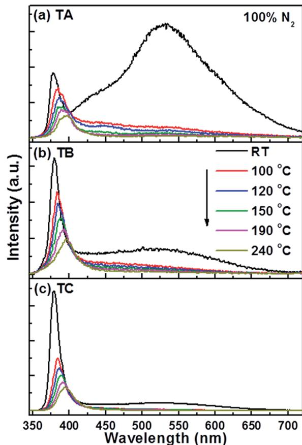
Fig. 3 PL spectra of (a) TA, (b) TB and (c) TC NR samples in 100% N<sub>2</sub> at various different temperatures in the range RT ≤ T<sub>NR</sub> ≤ 240 °C.
