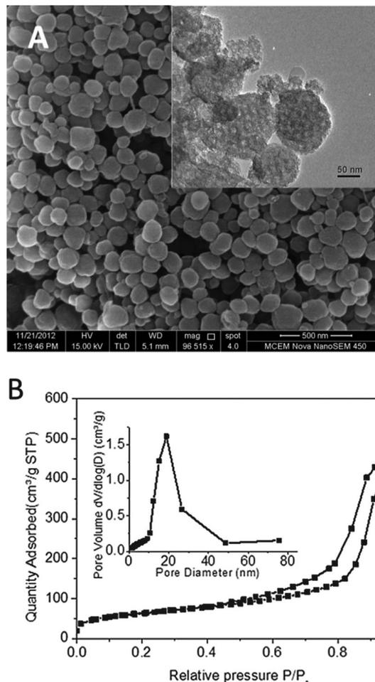
Fig. 1 (A) SEM image and TEM image (inset) of the large-pore mesoporous silica nanoparticles (LP-MSNs). (B) N<sub>2</sub> sorption isotherms and the inset BJH pore size distribution determined by nitrogen adsorption isotherm.
