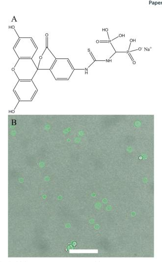
Fig. 5 (A) Chemical structure of Fluo-BP. (B) An overlay confocal micrograph of CaP capsules with Fluo-BP. Scale bar represents 50  $\mu m$ .
