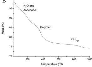
Fig. 3 (A) FTIR spectra of CaP capsules (red line), and CaP capsules annealed at 1000 °C (black line). (B) TGA curve of CaP capsules.
