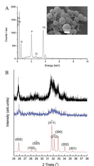
Fig. 4 (A) EDX spectrum and SEM micrograph of CaP capsules. (B) XRD patterns of CaP capsules as synthesized (blue line), CaP capsules annealed at 600 °C (black line), and simulated powder pattern of single crystal hydroxyapatite (red line).
