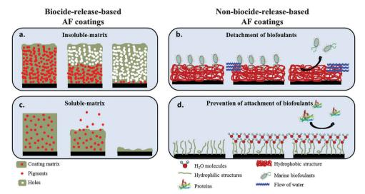
Fig. 2 Schematic of marine AF coating approaches: (a and c) Biocide-release based strategies; (b and d) non-biocide-release based strategies.
