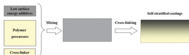
Fig. 5 Schematic of the formation of self-stratifying coatings.
