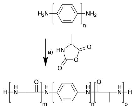
**Scheme 1** Synthesis of molecular tongue-twisters (oligoalanine-oligoaniline) from alanine *N*-carboxyanhydrides and amine-terminated oligoanilines. (a) DMF, Ar, 96 h. For tetraaniline-based MTT1,  $n = 2$ , and  $m + p \approx 10$ ; whereas for hexaaniline-based MTT2,  $n = 4$ , and  $m + p \approx 26$ .
