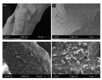
Fig. 5 SEM images showing HA formation on the surfaces of GCG coated 45S5 BG scaffolds after immersion in SBF for (a) and (b) 3 days and (c) and (d) 7 davs
