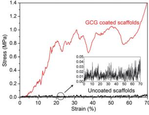
Fig. 6 Typical compressive stress-strain curves of uncoated and GCG coated 45S5 BG scaffolds, showing a remarkable improvement of mechanical properties by the presence of the GCG coating.
