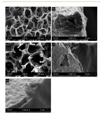
Fig. 1 SEM images of 45S5 BG scaffolds (a) and (b) before and (c)-(e) after coating with GCG.
