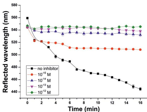
Fig. 6 Inhibition of the enzyme film with solutions of  $10^{-5}$  M acetylcholine and varying concentrations of the inhibitor as a function of the reflected wavelength. Each data point presents the average value of five measurements; the error bars indicate the standard deviation of these measurements.
