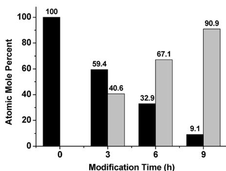
Fig. 5 Atomic mole percent of (Black) Au and (Grey) Si as a function of modification time, as determined from XPS analysis.
