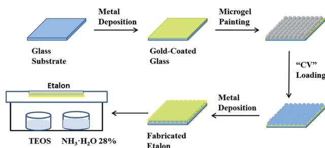
Fig. 2 Schematic showing the fabrication of the reservoir devices.
