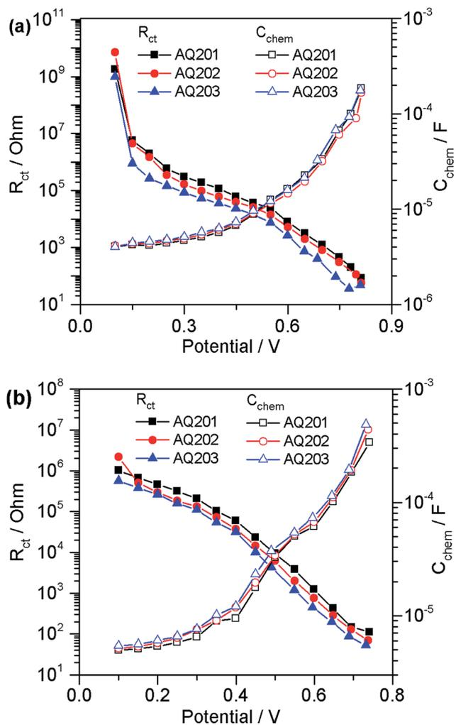
Fig. 5 Charge transfer resistance ( $R_{\text{ct}}$ ) and chemical capacitance ( $C_{\text{chem}}$ ) plotted against the IR drop corrected potential for DSSCs based on dyes AQ201, AQ202, and AQ203 with (a) the  $[\text{Co}(\text{bpy})_3]^{2+/3+}$  redox electrolyte and (b) the  $\text{I}^-/\text{I}_3^-$  redox electrolyte.
