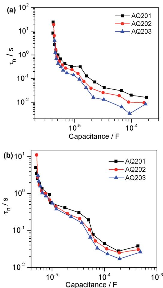
Fig. 6 Electron lifetime ( $\tau_n$ ) plotted against chemical capacitance ( $C_{\text{chem}}$ ) of DSSCs based on dyes AQ201, AQ202, and AQ203 with (a) the  $[\text{Co}(\text{bpy})_3]^{2+/3+}$  redox electrolyte and (b) the  $\text{I}^-/\text{I}_3^-$  redox electrolyte.
